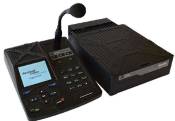
The network relies on specialized HF radios to communicate. Unlike most other radios that work in line of sight, HF radios can, in most conditions, work over hundreds or thousands of miles beyond line of sight. In fact, the HF technology used in UrgentLink is the same HF technology that U.S. Customs and Border Protection, the Office of the President and the U.S. military rely on for both primary and backup communications.<sup>7</sup>
