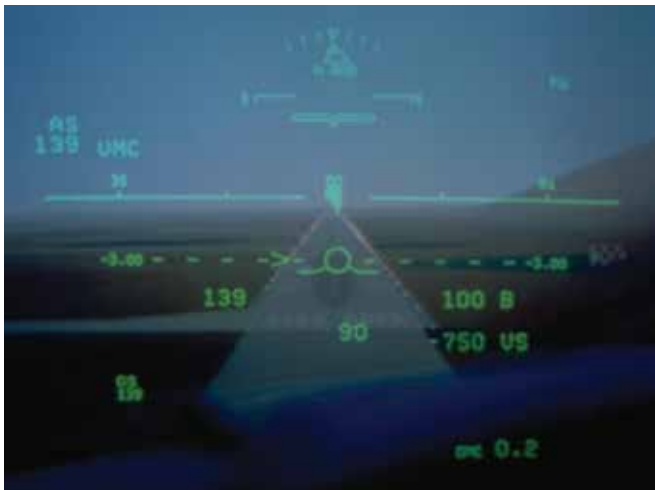
The flight path symbol makes flying a visual approach easy – even in a cross wind
